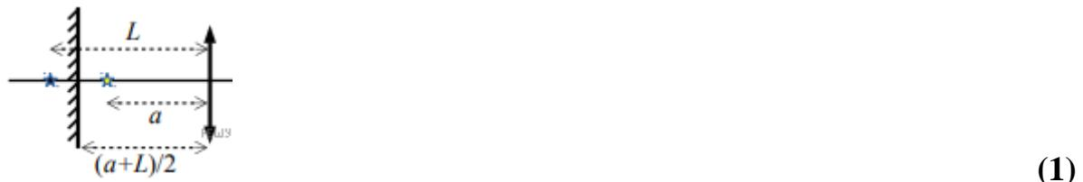
Such an image is obtained when light from an object hits a mirror without passing through the lens. It is easy to understand that the mirror should be on the same side of the lens as the object, and be located at a distance  $a=F$ :
